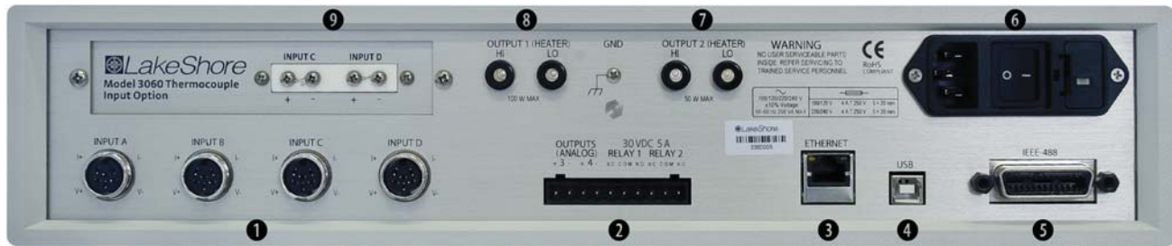
FIGURE 3-1 Model 336 rear panel
