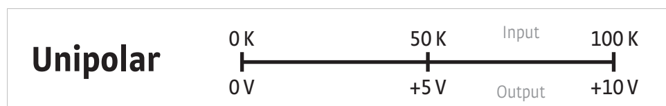
FIGURE 5-4 Output with polarity parameter set to unipolar
