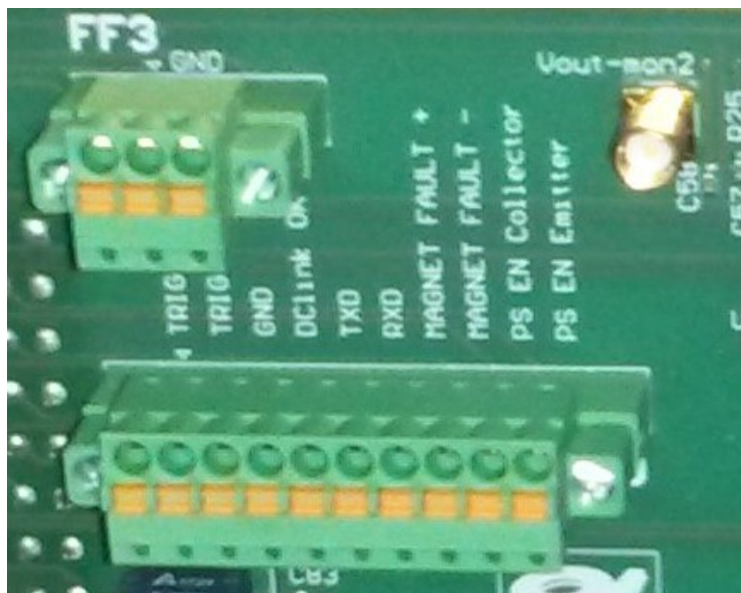
Figure 3: Interlock connector on A2720 backplane
